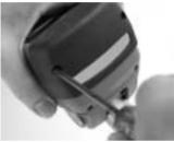
B. Open the battery pack by removing the cover.
